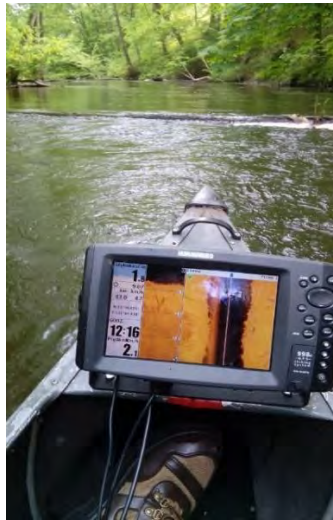
Figure 22. Echosounder Hummingbird SI 998c mounted on a boat. Photo: P. Parasiewicz, SSIFI.
