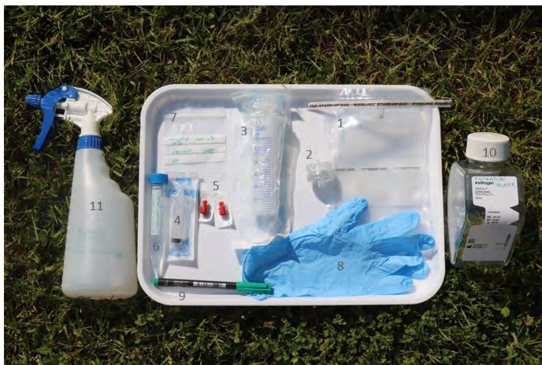
Figure 13. Sampling kit. The displayed kit contains the material needed to perform the proposed eDNA sampling in flowing water. (See Appendix 8.3 for a detailed list of suggested supplies, manufacturers, description and alternative suppliers. Source: AMBER D2.5.
