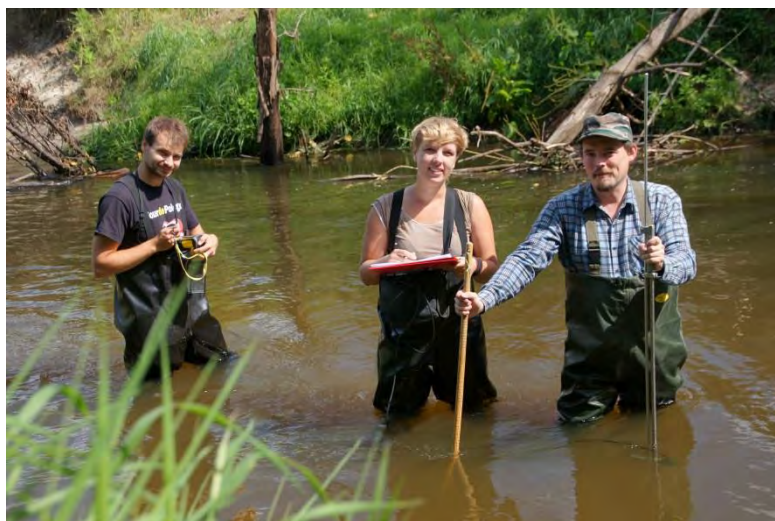
Figure 21. Measurement of velocities with electromagnetic flowmeter Marsh McBirney. Photo: J. Ligięza, SSIFI.
