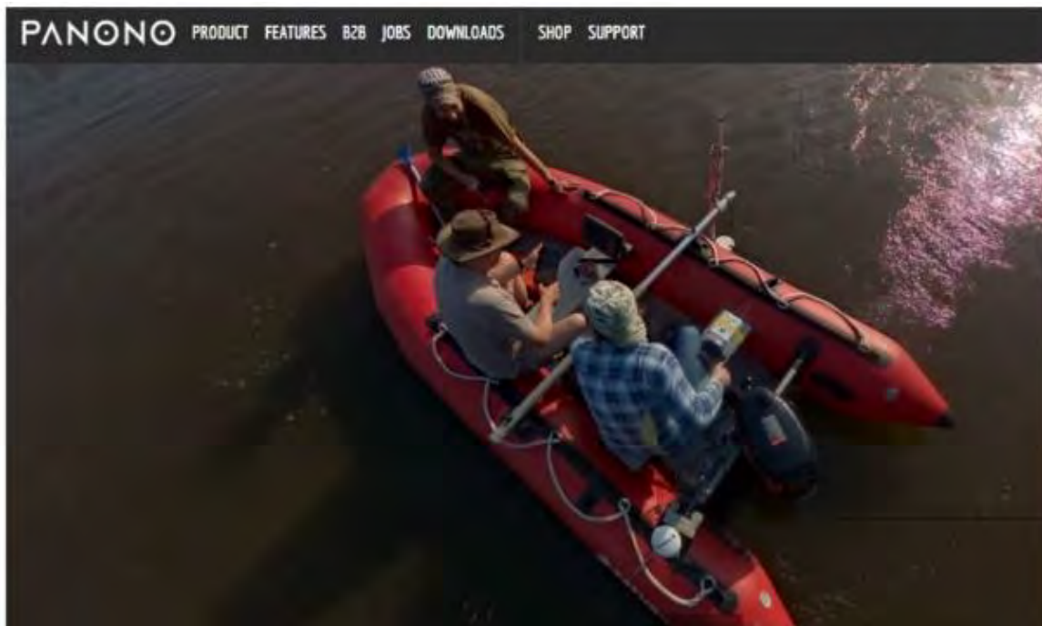
Figure 49. Hydraulic survey using Acoustic Doppler Profiler (mounted to the side) and side scan sonar and spherical camera. Photo: P. Parasiewicz, SSIFI.
