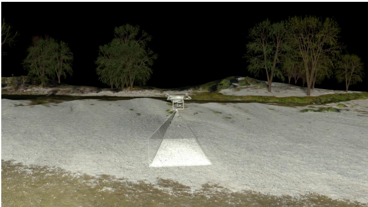
Figure 5. Schematic illustration of the Robotic Photosieving process. The drone is programmed to fly very low near the gravel bar in order to acquire highly detailed images of gravels that can be automatically sized. Collision avoidance systems and pilot control assure public safety.
