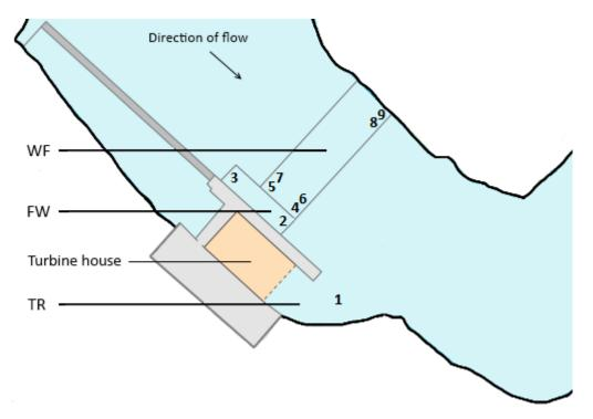
*Figure* **3**: Study site showing the turbine tailrace (TR, with antenna 1), bottom-baffle fishway (FW, antennas 2 and 3) and the Crump weir (WF, weir face; antennas 4 and 5 [controls right bank], 6 and 7 [tiled route] and 8 and 9 [controls left bank]).
